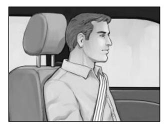
Slide the head restraint up or down so that the top of the restraint is closest to the top of your head. This position reduces the chance of a neck injury in a crash.
